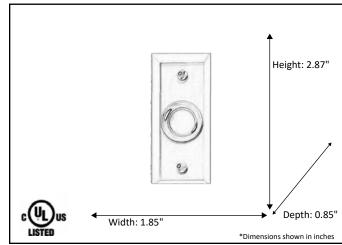
**ELECTRICAL REQUIREMENTS:** Fixture requires a door chime and transformer to lower voltage.
